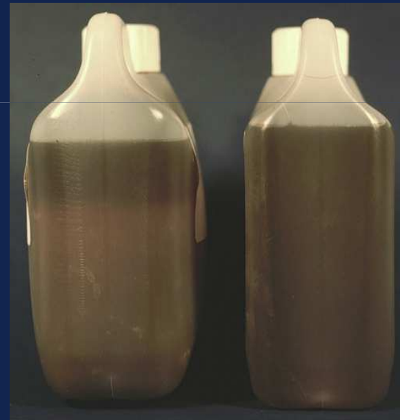
Container bulging from buildup of microbial CO 2
