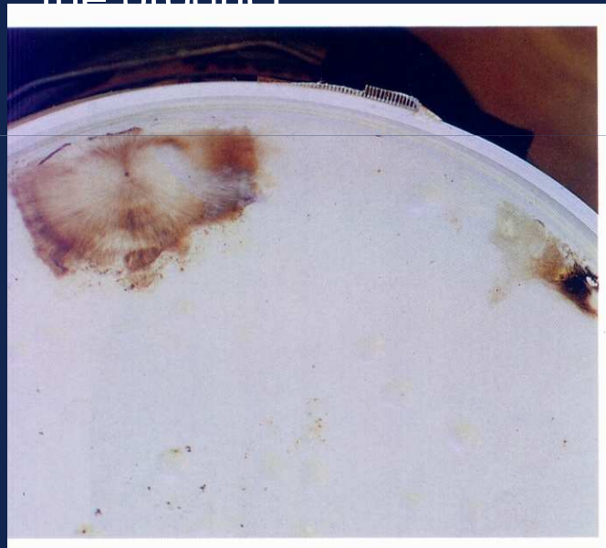
Fungal growth on surface of emulsion polymer
